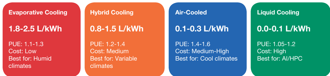
Figure 12: Water Usage Effectiveness (WUE) by Cooling Technology. Direct liquid cooling and air-cooled systems offer significant water savings compared to traditional evaporative cooling, an important consideration for deployment in water-stressed regions.
